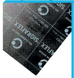
Graphite sheet (purity 98%) reinforced with a perforated stainless steel insert, specific gravity of graphite 1 gr/cm3 Universal material for chemical and petrochemical industries, suitable for thermal oils and steam, at high temperatures. Cryogenic temperatures up to +500°C in oxidising environments.
